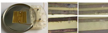
Fig. 10.2: Sample holder of UBremen with silicon gel mold material (left); device after ageing without (center) and with (right) scavenger.
