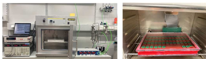
Fig. 10.4: Most recent weathering setup at TU Wien/KAI (left) with weathering cell (center). Schematic procedure of standard preparation and measurement for LA-ICP-MS calibration enabling quantitative analysis.
