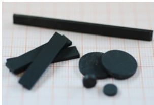
Fig. 1: Specimens prepared from the bulk ferrite ceramic.
