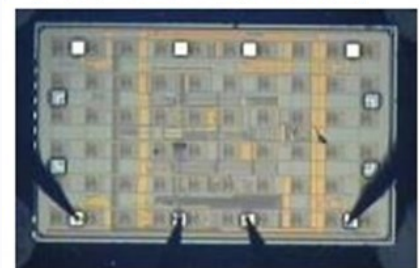
Measurement principle: n & pMOS current mirrors.
